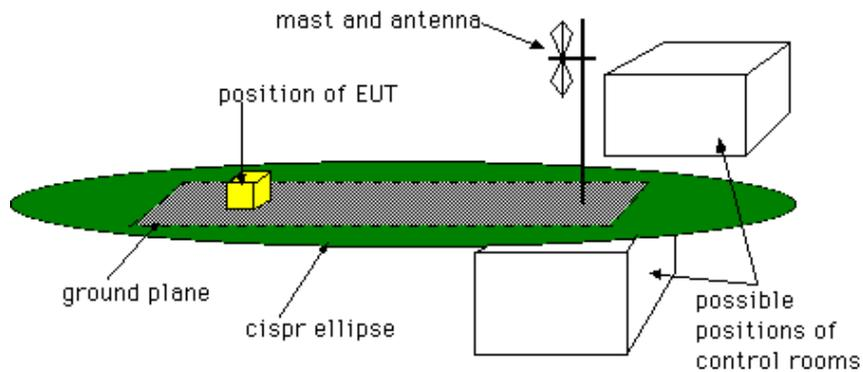
The antenna height should be remotely adjustable from 1m to 4m. Measuring instrumentation should be outside the ellipse at the position shown or in a room under the ground plane.
