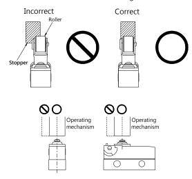
•To operate switch in accordance with direction of the switch button, please press the switch button vertically
