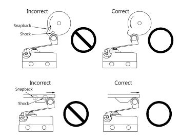
•Avoid uneven weight on the switch lever while operation. Part of actuator wear off can lead to internal structures damaged and decreased reliability.
