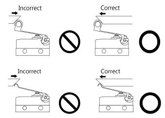
•Set the cam and plunger angles from the range of 30° to 45°  $^{\circ}$  If angle is over this range, the horizontal stress will be applied to the lever.
