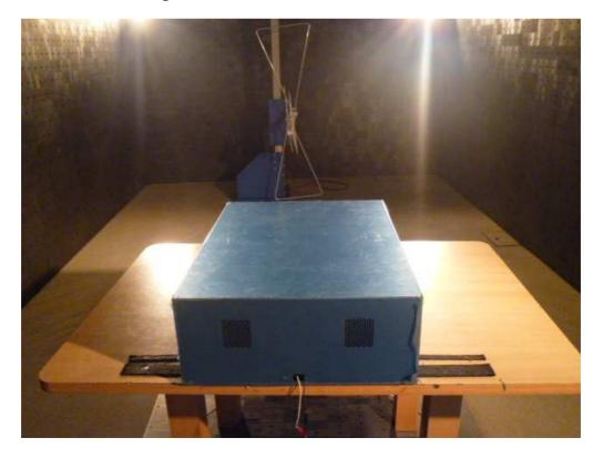
\*During the radiated test, the power-supply has to test with chassis, which is not allowed to be operated stand-alone. (For user, final assembly has to comply with corresponding EMC-and safety-regulations.)
