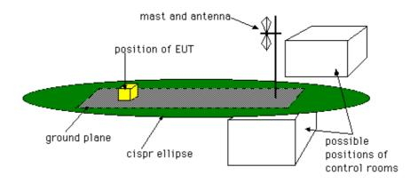
The antenna height should be remotely adjustable from 1m to 4m. Measuring instrumentation should be outside the ellipse at the position shown or in a room under the ground plane. The whole or part of the site may be enclosed in an RF transparent building. For precompliance testing a 3m test site with a fixed height antenna (at 1.5-2m height) and no metallic ground plane may be used. This may be a clear area on a car park or a grass area but should
