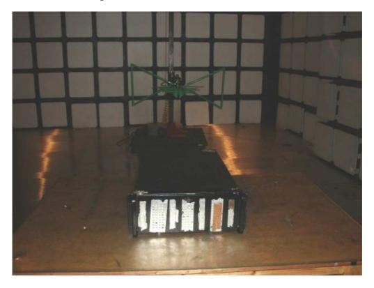
\*During the radiated test, the power-supply has to test with chassis, which is not allowed to be operated stand-alone. (For user, final assembly has to comply with corresponding EMC-and safety-regulations.)
