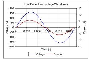
Input AC Current Waveform (ITHD = 8.98%, 50% Load)
